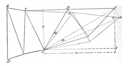
Let the truss represented in the sketch above be fixed at A and B. If any member, for instance CD, elongates,  $\Delta$  denoting the increment, then that portion of the truss which is influenced by the elongation of that member will rotate around a point E, which point will be found by
