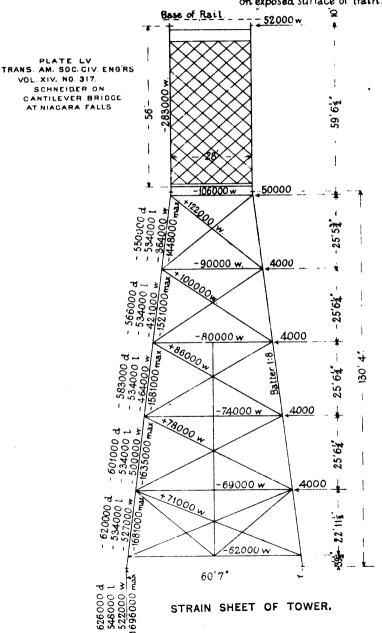
The tower-posts, lower chords, center and end-posts of cantilevers, pins and top-castings for towers are of steel; all the other parts of the bridge are of wrought-iron, excepting the shoes for the tower-posts, filling rings, washers and hand-rail posts, which are of cast-iron.
