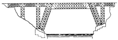
4. The recommended design was a braced arch, hinged in the center
