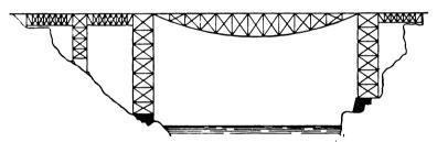
3. The third design was similar to No. 2, except that the length of the central span was reduced from 430 feet to 300 feet by leaning towers, somewhat like the false works of the Attock Bridge, in India, lately illustrated in London *Engineering*. The estimated weight of this design was 2 590 tons. This design is only eclipsed in ugliness by Max Am Endes' bridge in South Africa.
