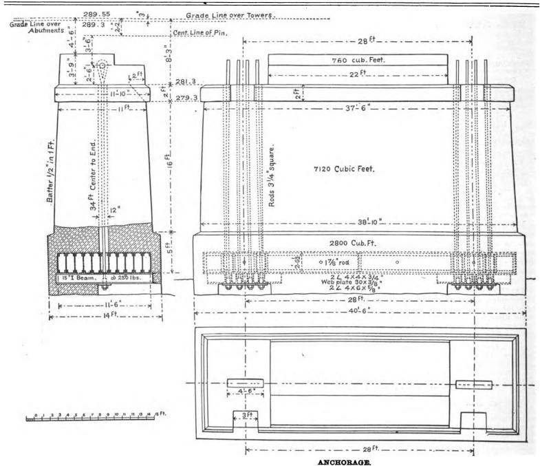
The shore ends of the cantilevers are attached to short links revolving on pins anchored to the masonry; these links serve as rockers and allow for the expansion and contraction of the shore ends of the cantilevers. Expansion joints are also provided for at the connection of the intermediate span with the river ends of the two cantilevers, the intermediate span being suspended from the extreme ends of the river arms.
