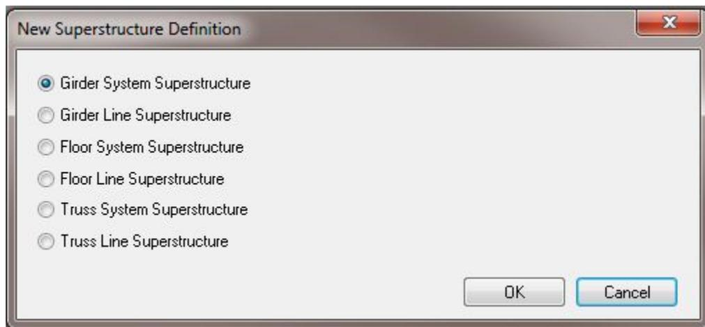
Select **Girder System Superstructure** and the Structure Definition window will open. Enter the data shown below:
