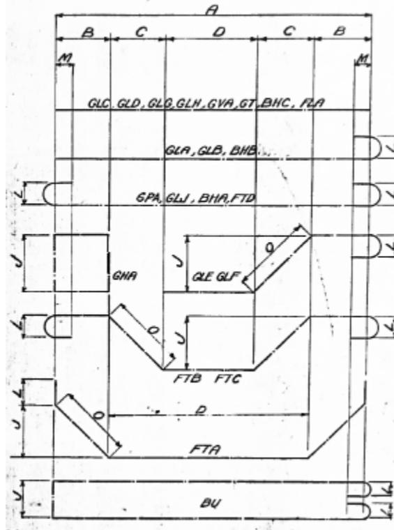
**Description and Bending Details of Longitudinal Girder Reinforcing Steel**
