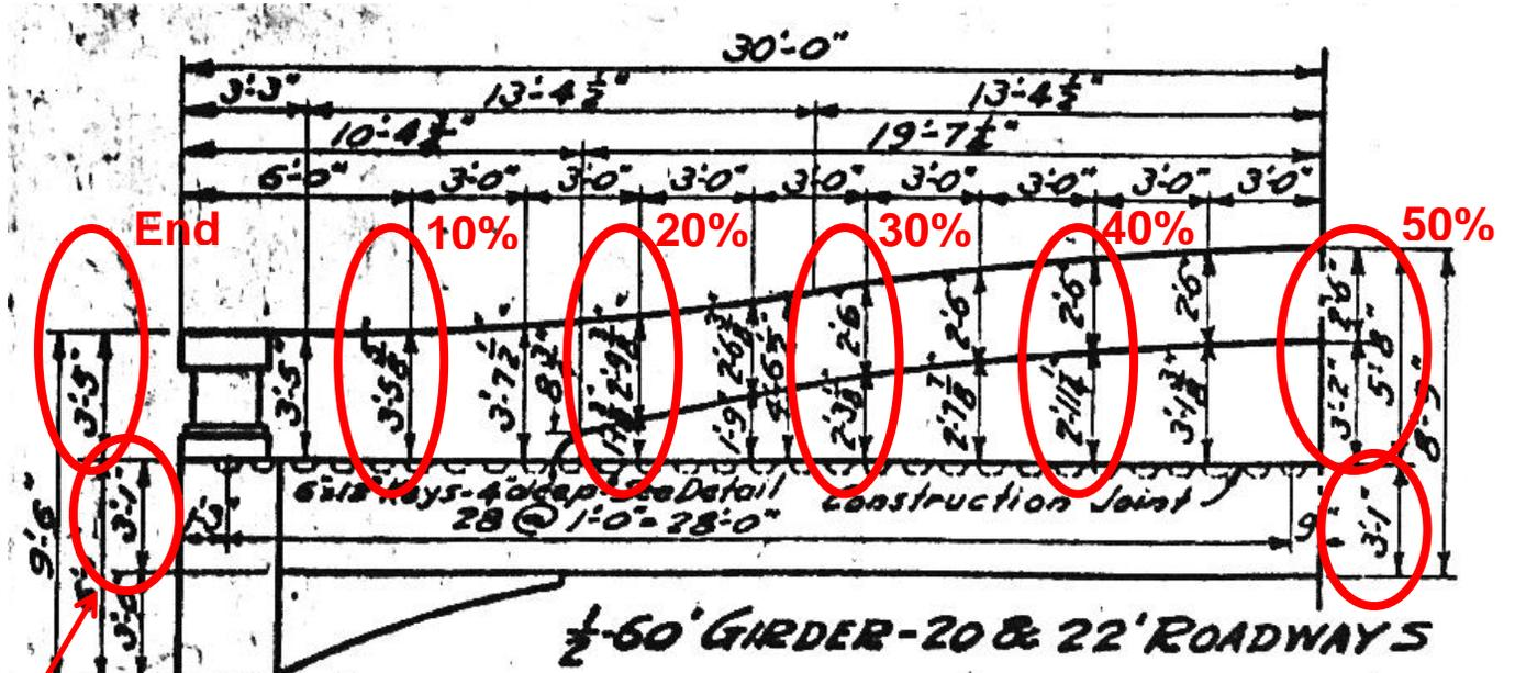
Elevation showing dimensions of the top flange/web at various cross sections
