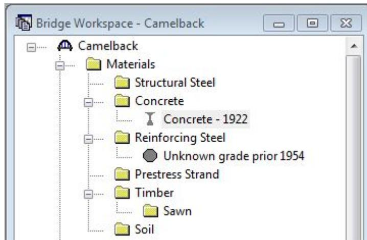
To add a new concrete material click on **Concrete** in the tree and select *File/New* from the menu (or right mouse click on **Concrete** and select *New*).
