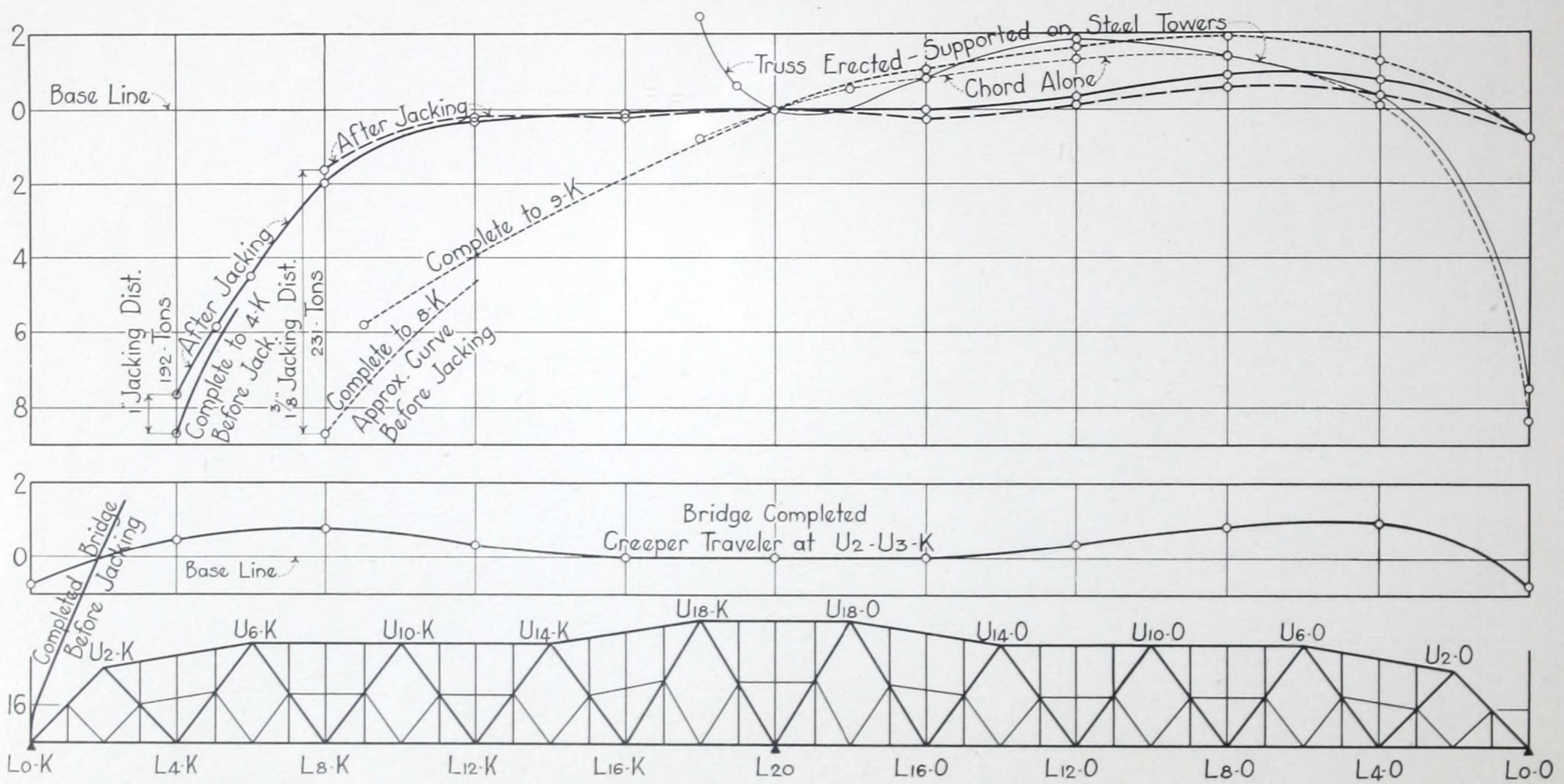
Curves of lower chord under various erection conditions.
