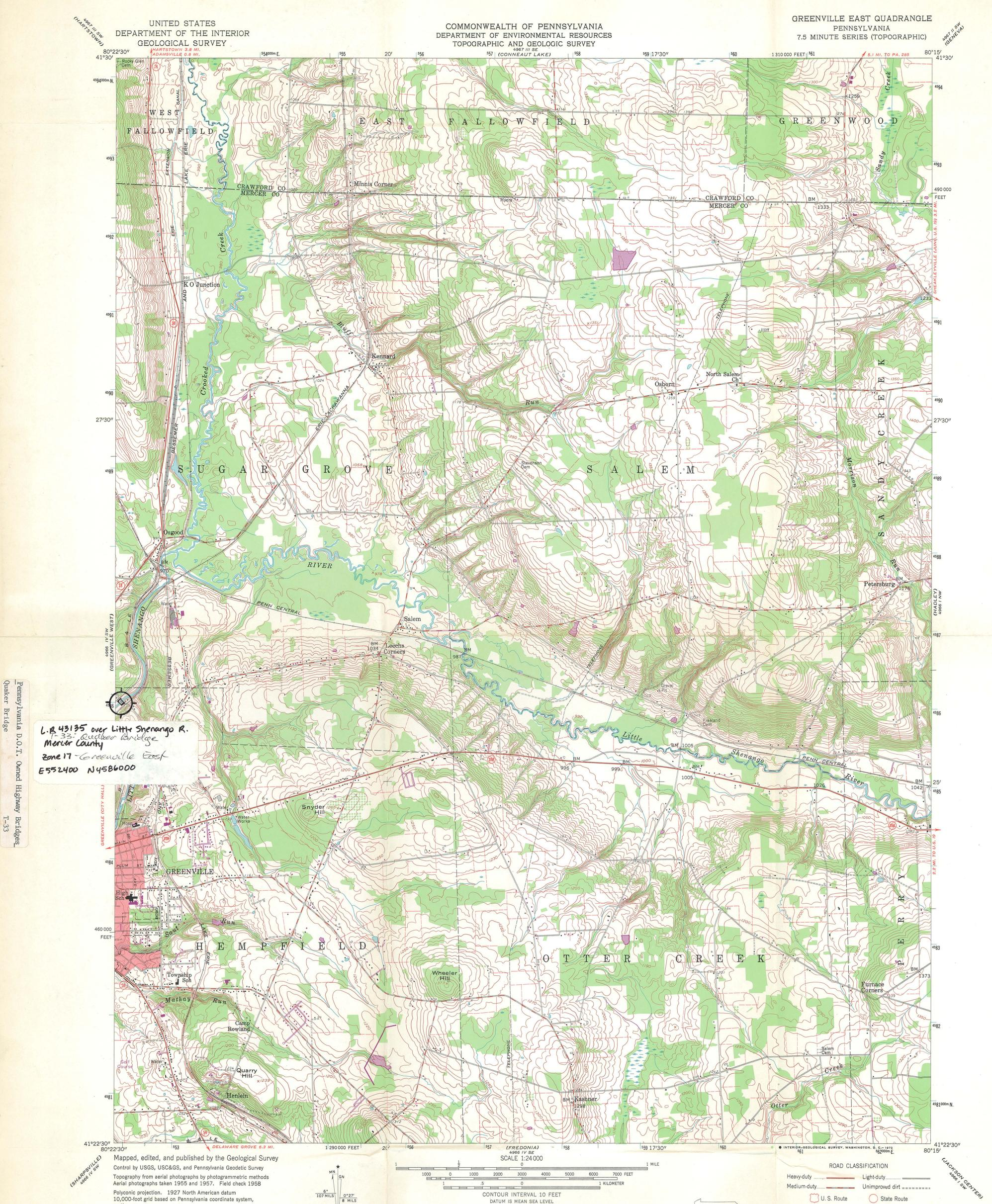
Polyconic projection. 1927 North American datum 10,000-foot grid based on Pennsylvania coordinate system, north zone 1000-meter Universal Transverse Mercator grid ticks, zone 17, shown in blue
