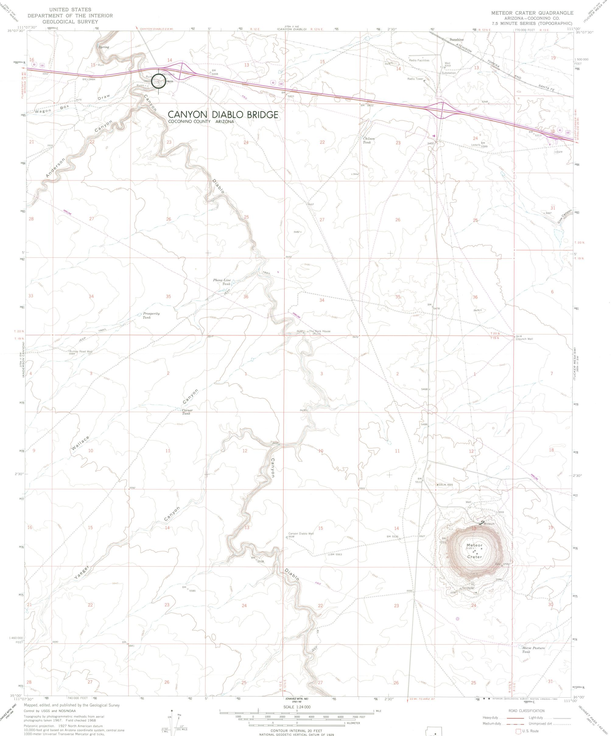
lyconic projection. 1927 North American datum 10,000-foot grid based on Arizona coordinate system, central zone 1000-meter Universal Transverse Mercator grid ticks, zone 12, shown in blue To place on the predicted North American Datum 1983 move the projection lines 1 meter north and 63 meters east as shown by dashed corner ticks Fine red dashed lines indicate selected fence lines
