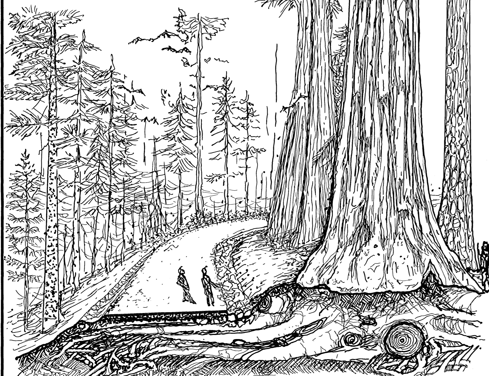
Road Section showing relationship to Sequoia Root System Bats use fly space over Roadway
