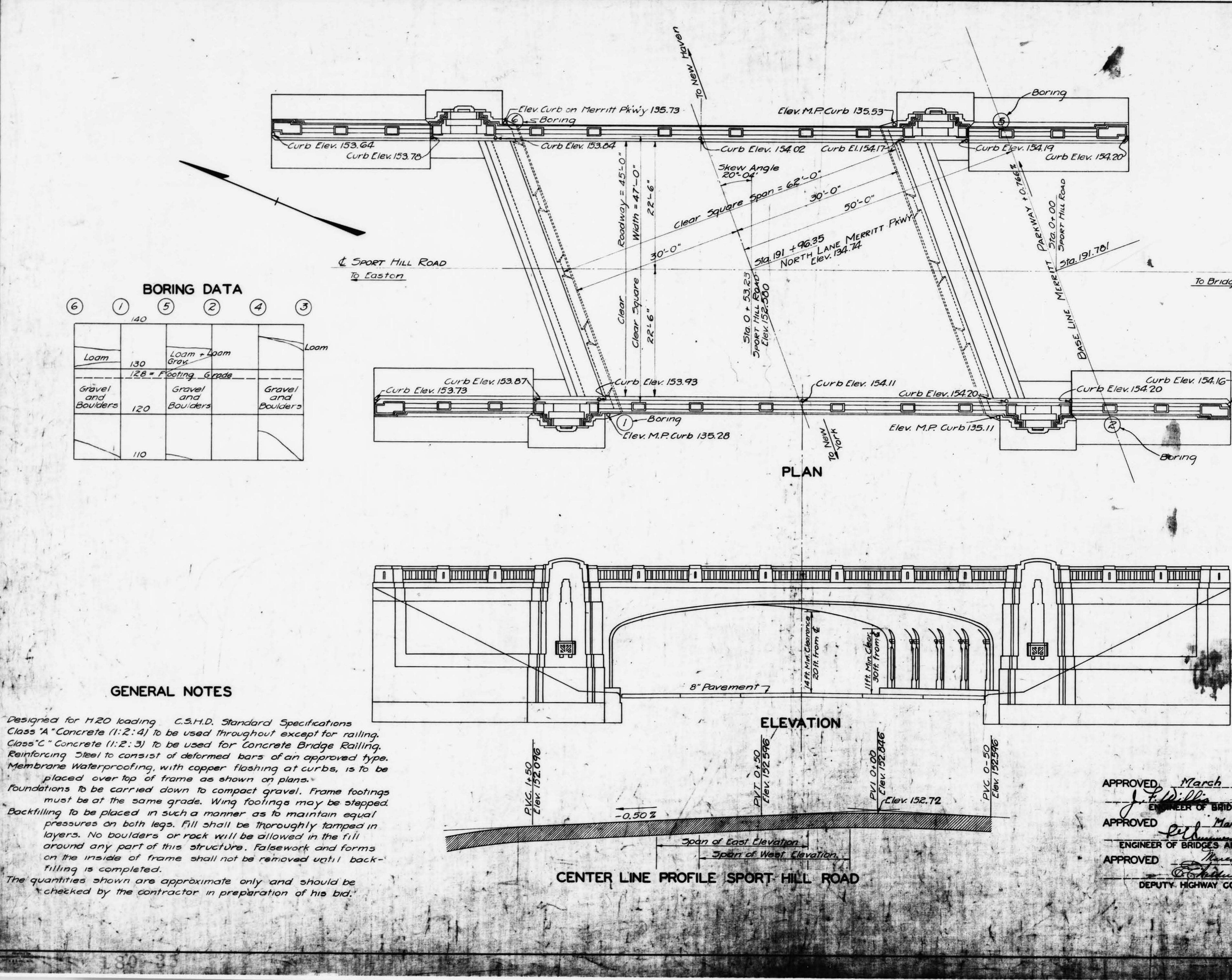
Class "A" Concrete (1:2:4) to be used throughout except for railing. Class" C" Concrete (1:2:3) to be used for Concrete Bridge Railing. Reinforcing Steel to consist of deformed bars of an approved type. Membrane Waterproofing, with copper flashing at curbs, is to be placed over top of frame as shown on plans.
