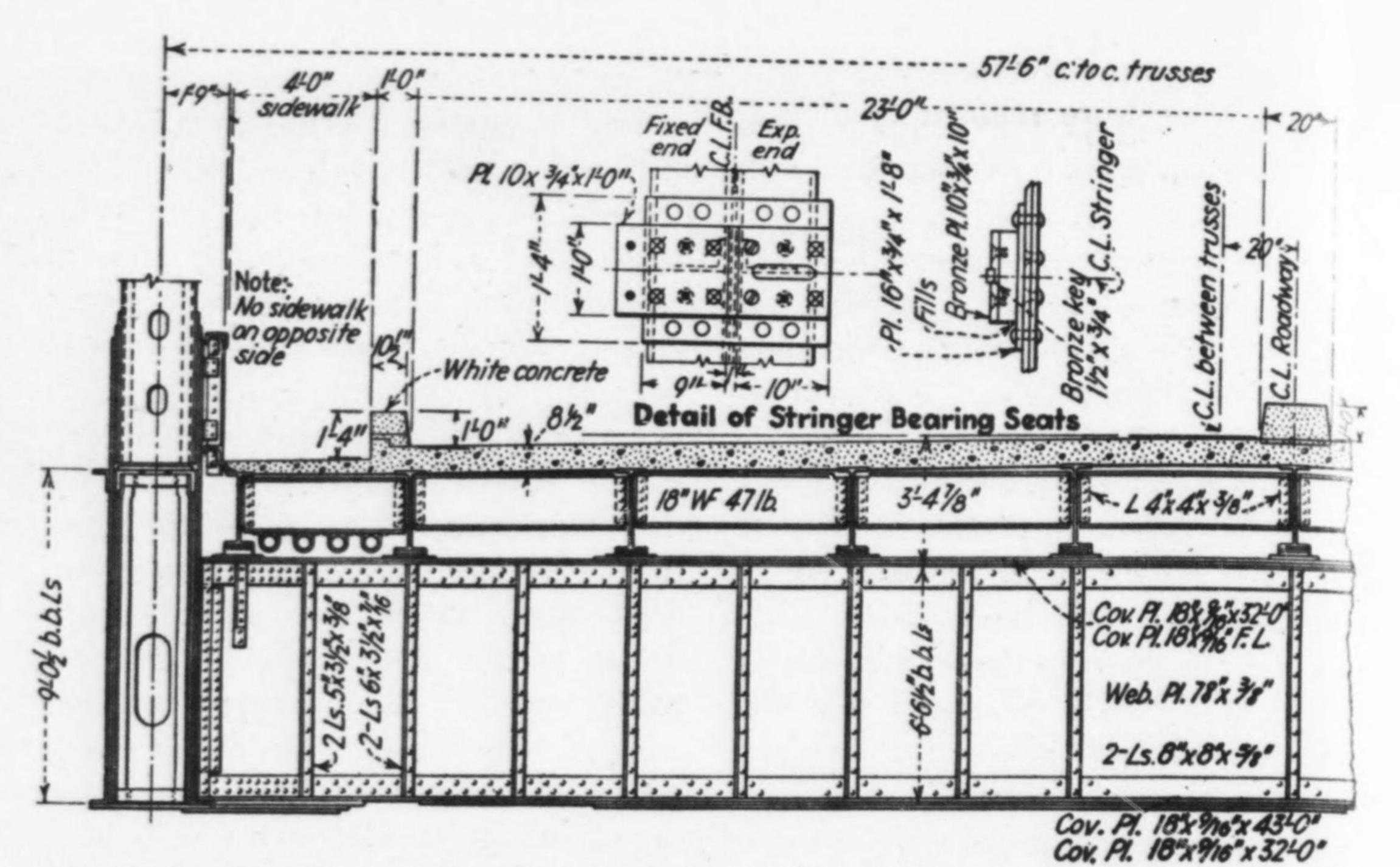
Fig. 3. Cross-section of deck of St. Georges tied arch. The solid concrete deck contributes desirable stiffness. One end of each stringer is on an expansion bearing to avoid floorbeam distortion.
