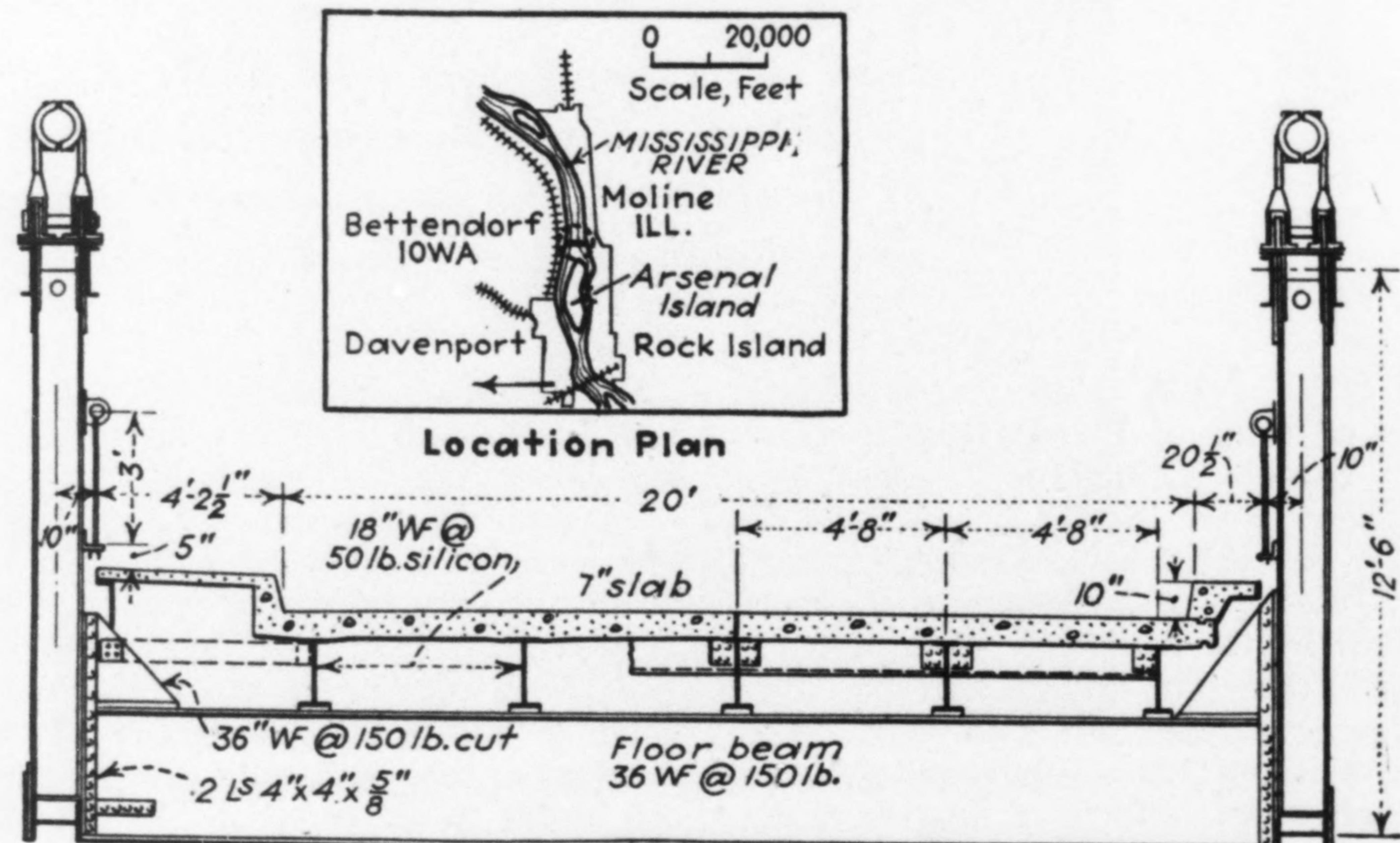
Suspended Span Section
