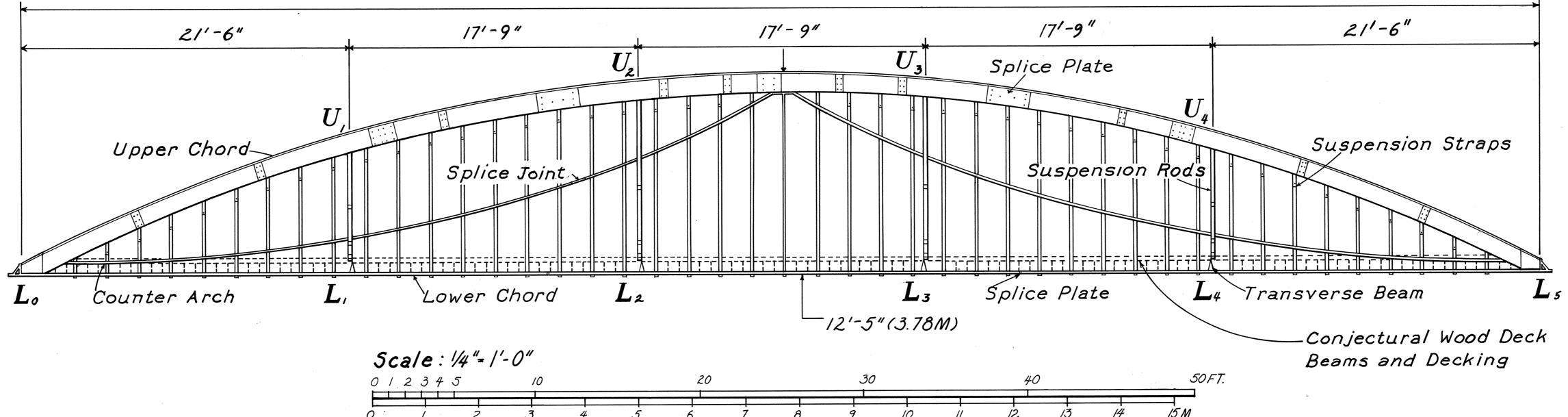
The Upper Pacific Mills Bridge, built in 1864 to carry workers and supplies to the upper and lower Pacific Mills in Lawrence Massachusetts, is a single-span tied arch and one of only two known surviving examples of the wrought-iron tubular arch bridges built by Thomas W. H. Moseley. First built in 1855, Moseley's designs evolved over a period of approximately 20 years and were the subject of several U.S. patents.
