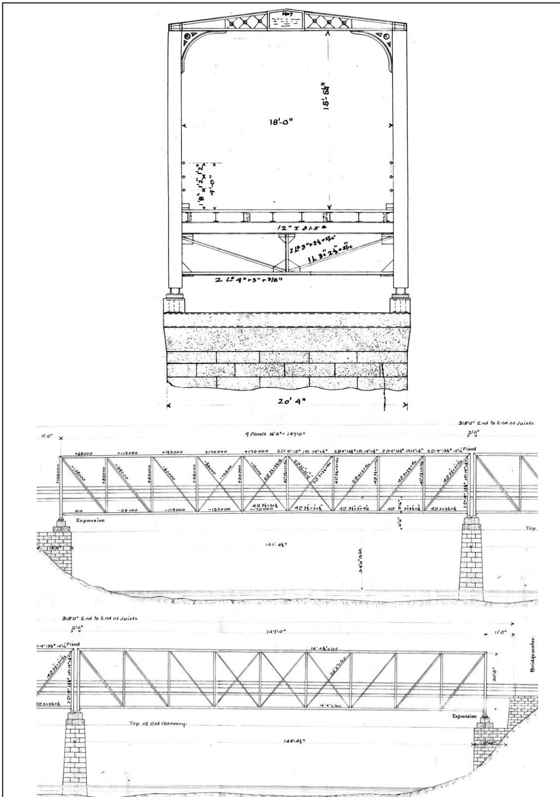
FIGURE 3: Ashland-Bridgewater, 076/080 over Pemigewasset River. An uncommon two-span, half-through, Pratt truss with vertical end posts. Designed by John Storrs and built by United Construction Co. in 1907. Replaced in 1937. Original plan drawings by John Storrs, 1907 (NHDOT Plan files).
