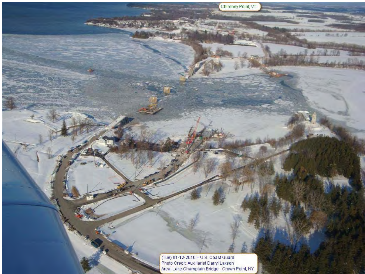
Figure 75. Aerial view of the demolished Lake Champlain Bridge, looking north from the Crown Point State Historic Site, January 12, 2010. The truss spans are underwater, while the viaduct spans on either end remain standing. Photograph by U.S. Coast Guard Auxiliarist Darryl Laxson.
