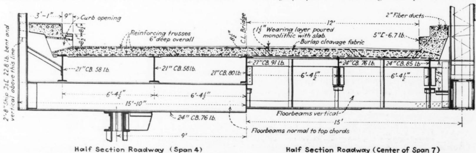
FIG. 4—TYPICAL CROSS-SECTIONS OF DECK
