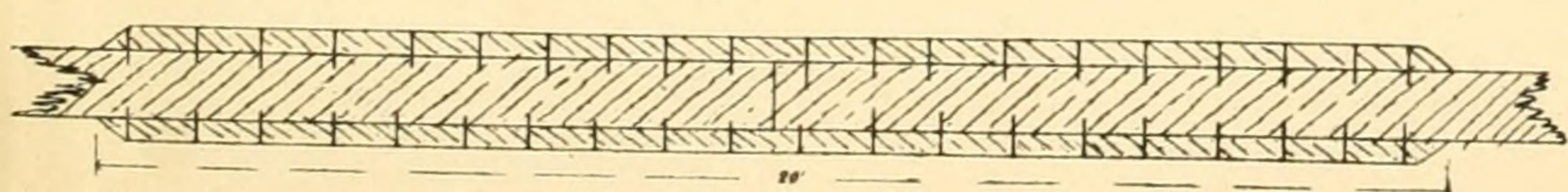
*Plan showing Method of Splicing Piles.*
