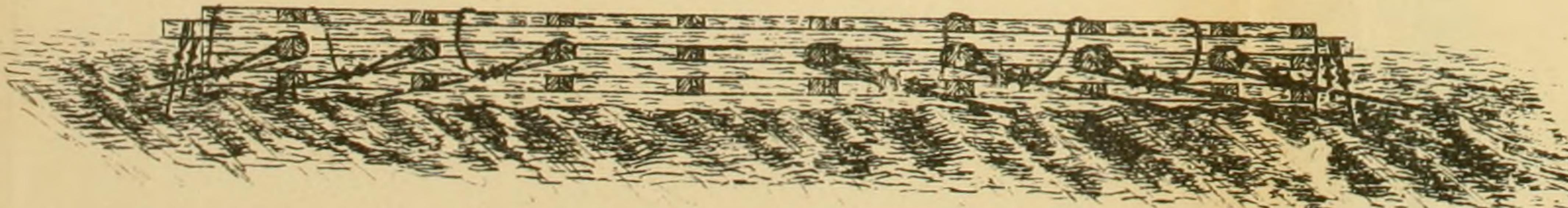
CRIB, ANCHORED IN POSITION
