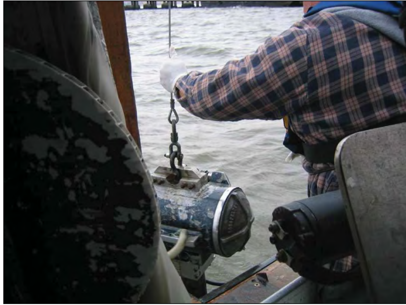
Figure 4. Vibracore being lowered over the side of research vessel.
