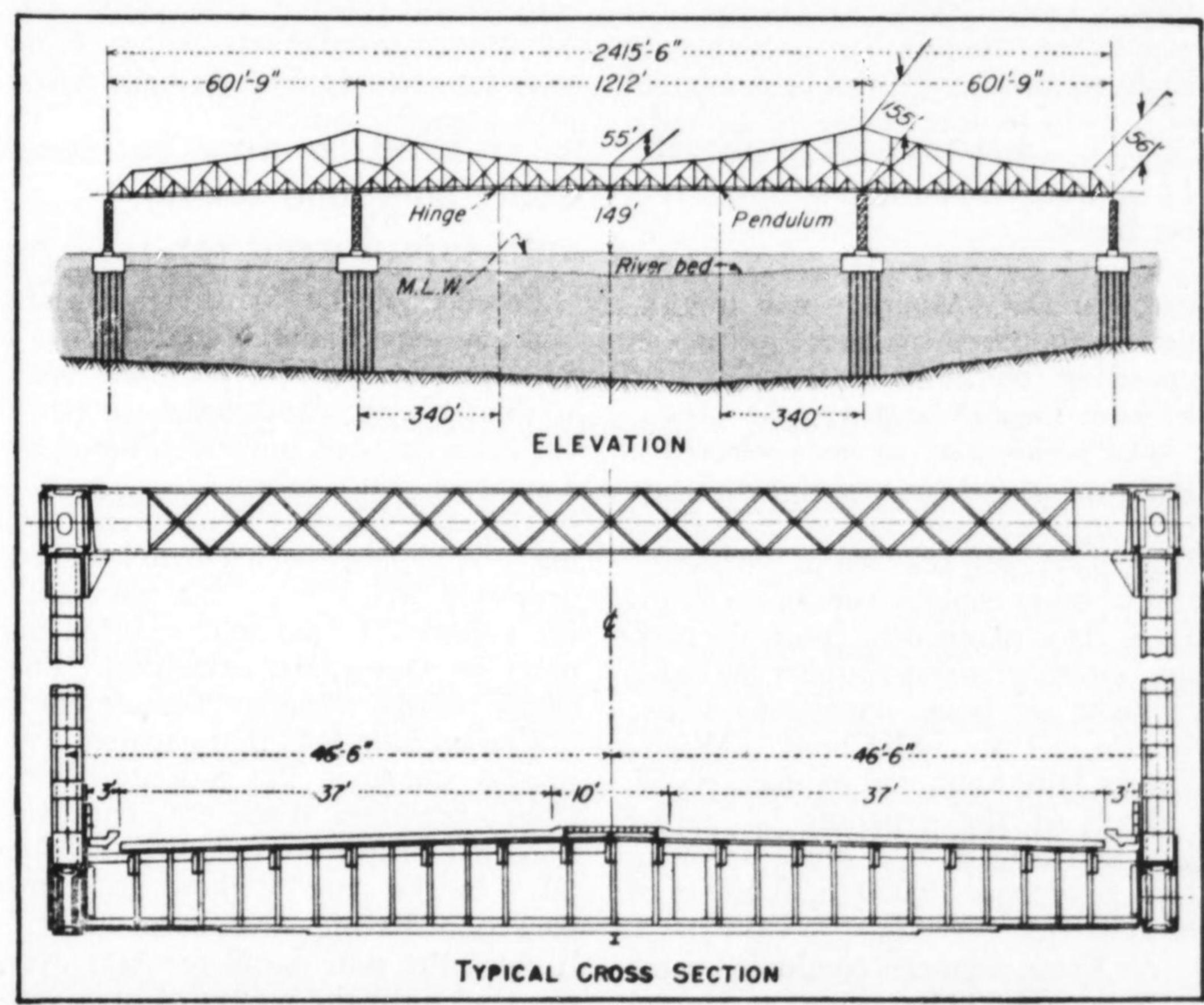
CANTILEVER TRUSSES will carry the New York State Thruway over the main channel of the Hudson River. Foundations are hollow concrete-caissons on piles.
