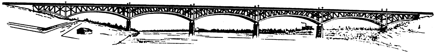
FIG. 17—KNOXVILLE ARCHED CANTILEVER.
