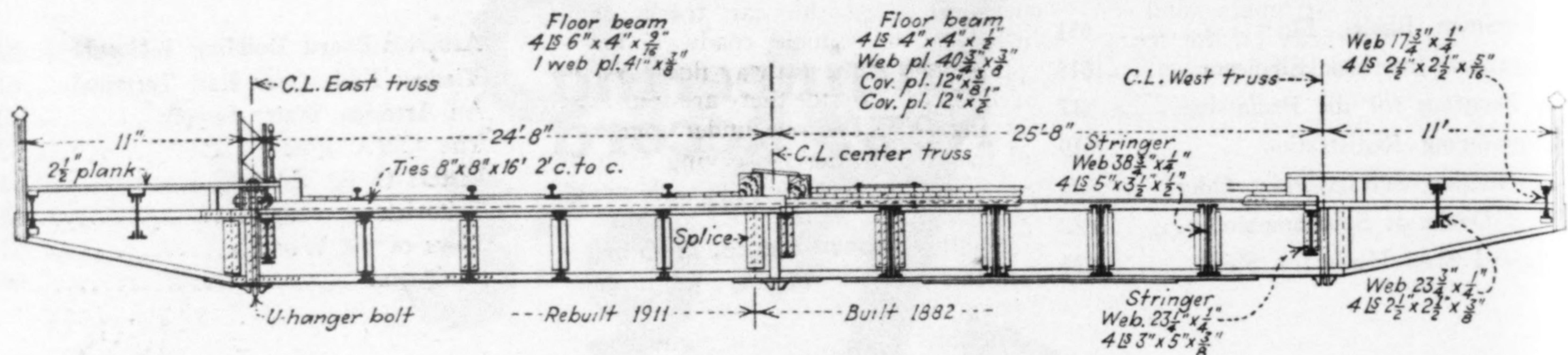
Fig. 2—Old wrought-iron and steel floor, with 11-in. timber decking for vehicle roadway.
